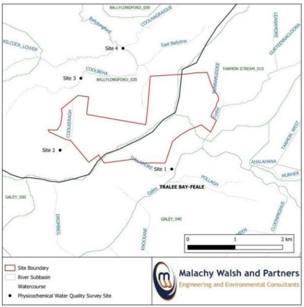
Figure 6-1: Physicochemical water quality sampling points.
