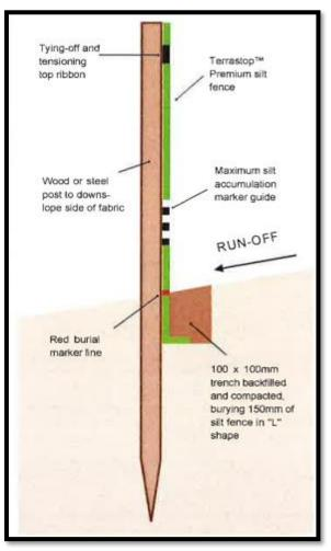
Figure 6-12: Schematic Detail of a Silt Fence
